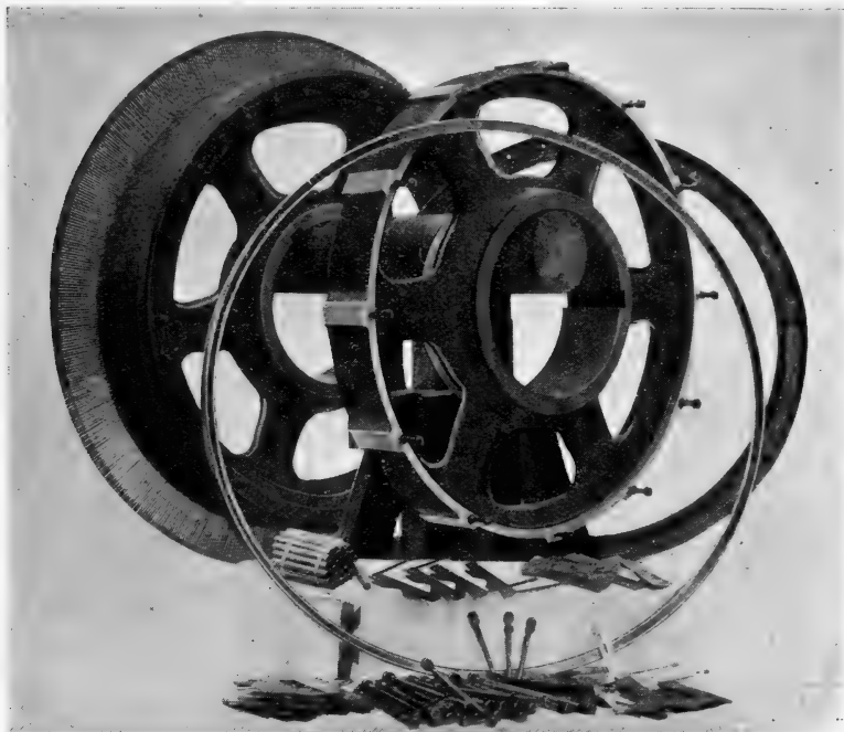
FIG. 138.—Component parts of large Commutator. Dick, Kerr & Co.
